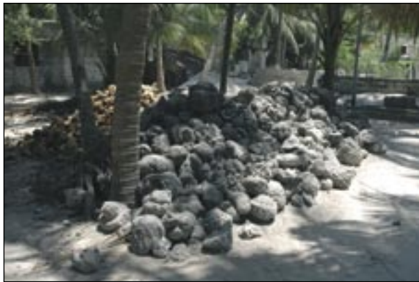
Figure 3. Coral boulders collected for construction. Both live and dead colonies are broken off the reef using iron rods. Photo: JERKER TAMELANDER.
