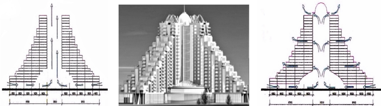
Figure 1a – Design of "Tau Samal" multifunctional residential complex at the intersection of Zhandosov and Navoi Streets. Changes in the aeration of the central building, depending on the upper floor structure of the atrium
