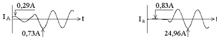
Figure 4 – The results of the simulation of currents in the phase A windings in the transformer of TSZI-6 type in event of a three-phase short circuit at the secondary winding end
