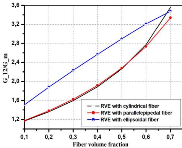
**Figure 6. In-plane shear modulus with respect to fiber volume fraction for different geometrical configurations of fiber.**
