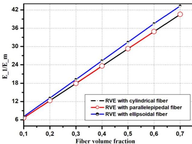
*Figure 4. Longitudinal Young's modulus with respect to fiber volume fraction for different geometrical configurations of fiber.*
