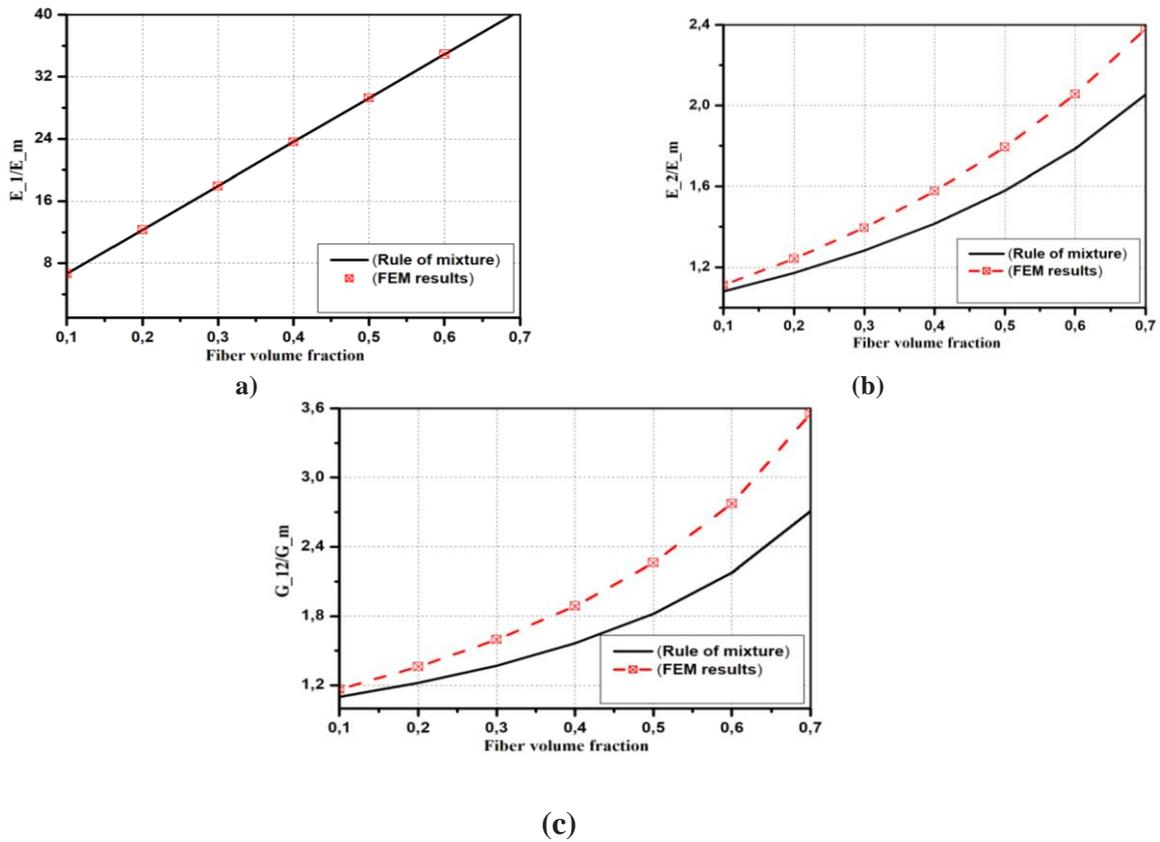
Figure 2. Validation of the computed elastic properties with different fiber volume fraction -a/ Longitudinal Young's modulus -b/ Transverse Young's modulus -c/ Shear modulus
