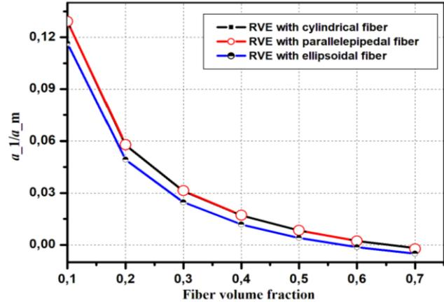
**Figure 7. Longitudinal coefficient of thermal expansion with respect to fiber volume fraction for different geometrical configurations of fiber.**
