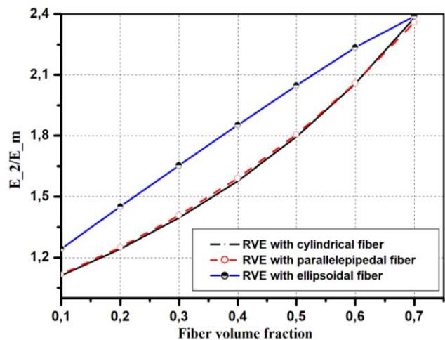
*Figure 5. Transverse Young's modulus with respect to fiber volume fraction for different geometrical configurations of fiber.*
