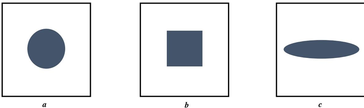
Figure 1. Representative volume element of cases of study where the characteristic dimension of fiber of each case is:
