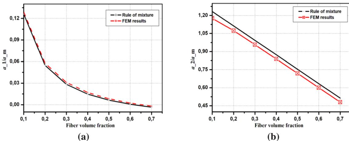
Figure 3. Validation of the computed coefficients of thermal expansion with different fiber volume fraction -a/ Longitudinal Coefficients of thermal expansion -b/ Transverse Coefficients of thermal expansion
