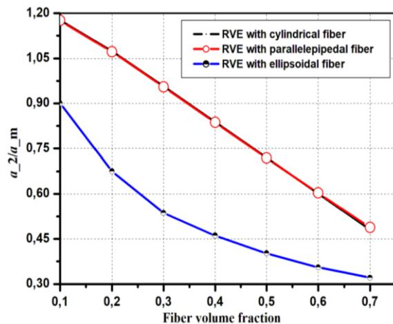
**Figure 8. Transverse coefficient of thermal expansion with respect to fiber volume fraction for different geometrical configurations of fiber.**
