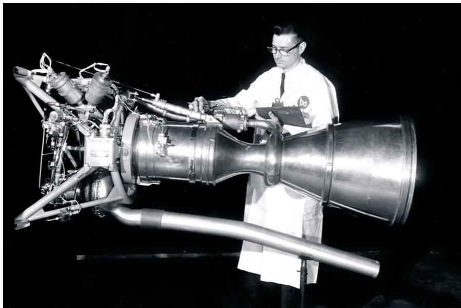
Figure 3. Model 8096 Agena engine with two cartridge starters, Bell Agena Collection. Niagara Aerospace Museum
