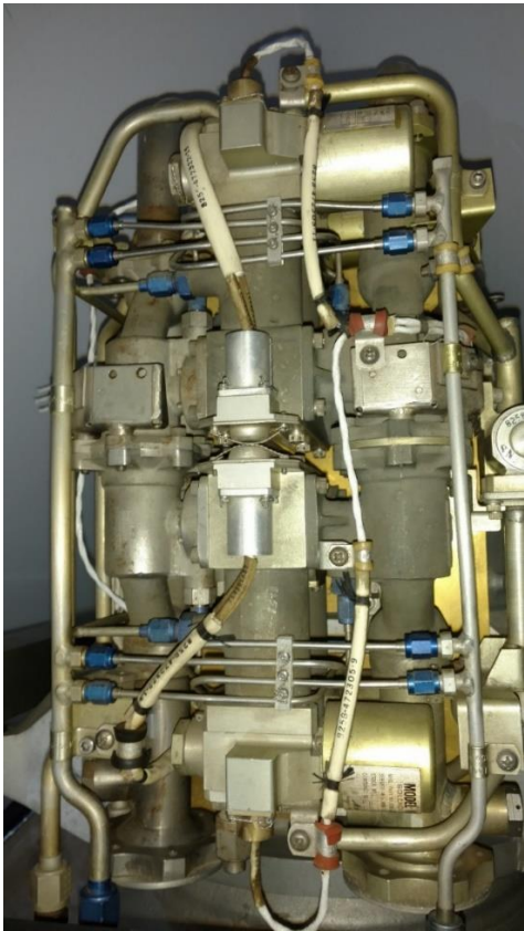
Figure 10. LMAE Control Valve Manifold. Niagara Aerospace Museum
