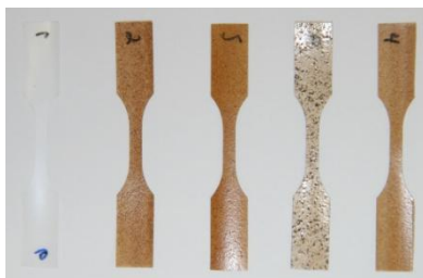
Fig. 6 Photograph of films. From left: Pure LDPE, LAP 150°C, LAP 160°C, LAP 170°C and LAP 150°C pre-blend.
