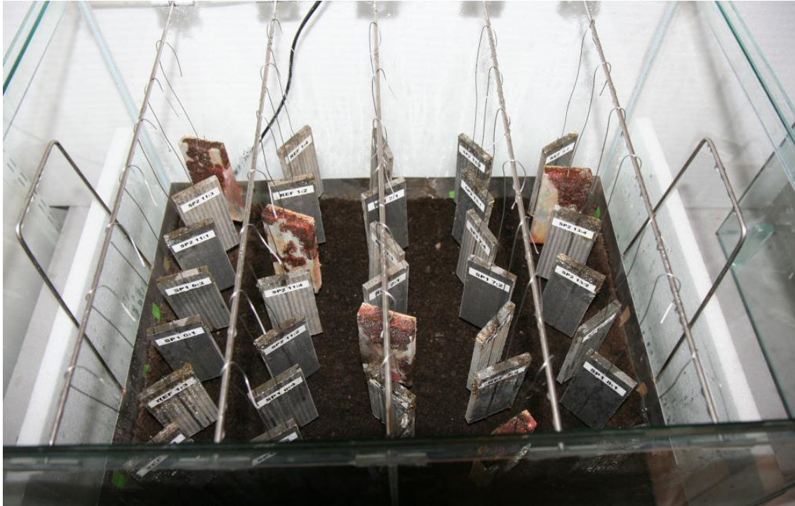
Fig. 1. Specimens suspended in the environmental chamber.
