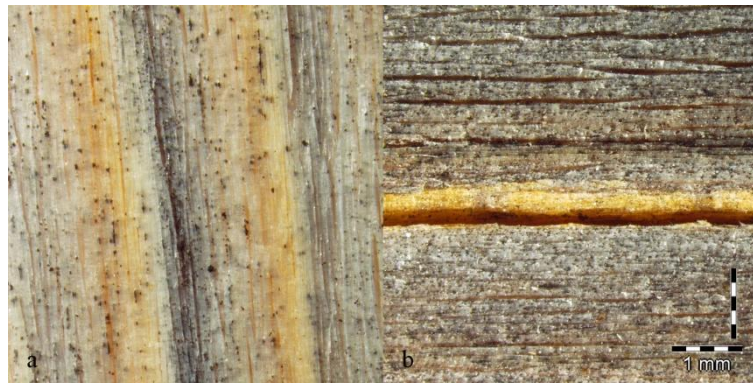
Fig. 7. Norway Spruce, annual rings horizontally (a) and vertically (b) oriented, east exposure 1322 days.
