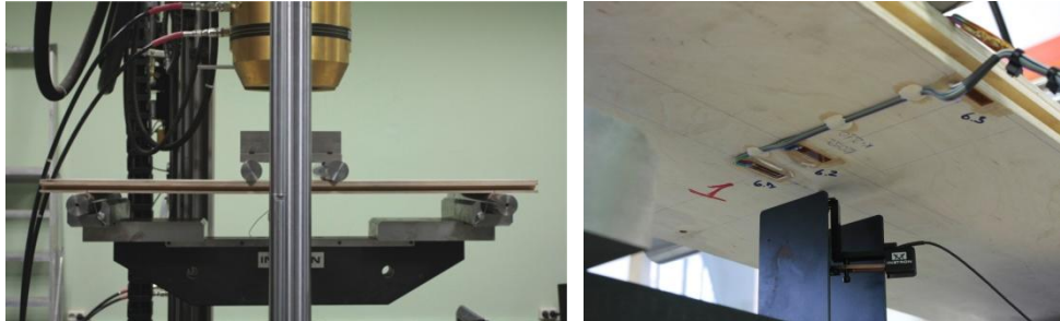
Fig. 2. Experimental 4-point bending set-up according EN 789.
