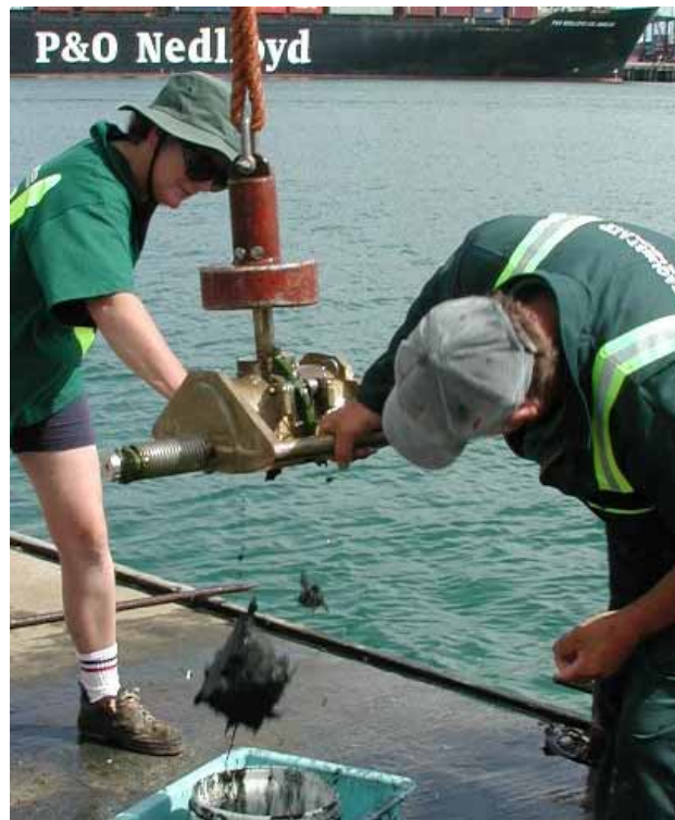
Figure 8: Shipek grab sampler: releasing benthic sample into bucket
