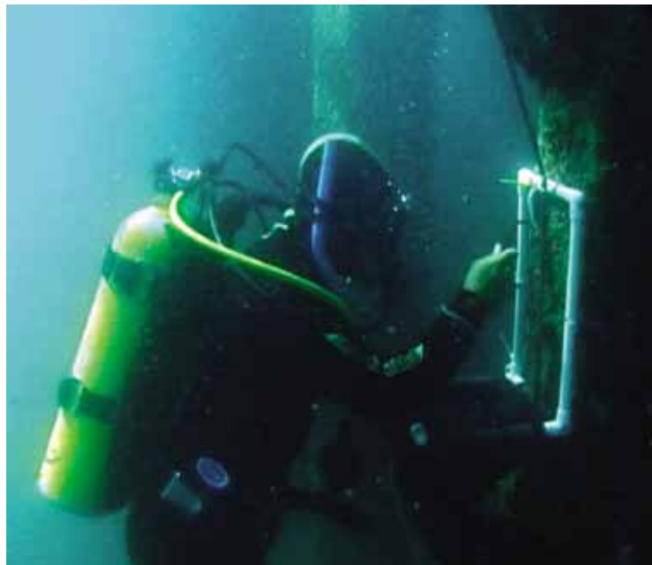
Figure 7: Diver sampling organisms on pier piles.
