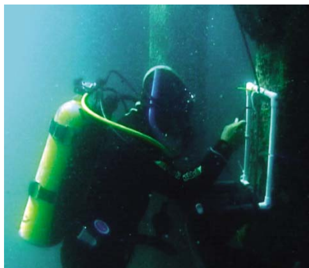
Figure 3: Diver sampling organisms on pier piles.
