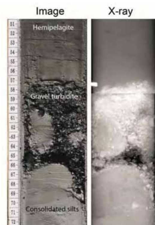
Figure 4-4: True colour image and x-ray radiograph of a core from Cook Strait Canyon. TAN1613-05 (Cook 2) showing consolidated silts overlain by a gravelly turbidite and hemipelagite.
