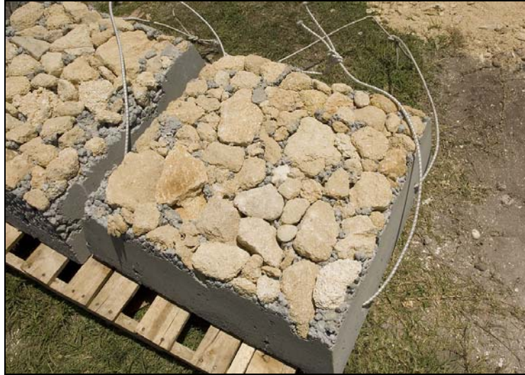
Figure 8.3. Prototype mitigation reef modules made from articulated mat with integral coquina rock surface. Each block is about 30 inches x 30 inches x 12 inches (Continental Shelf Associates, Inc. et al., 2006). Photo by D. Snyder.
