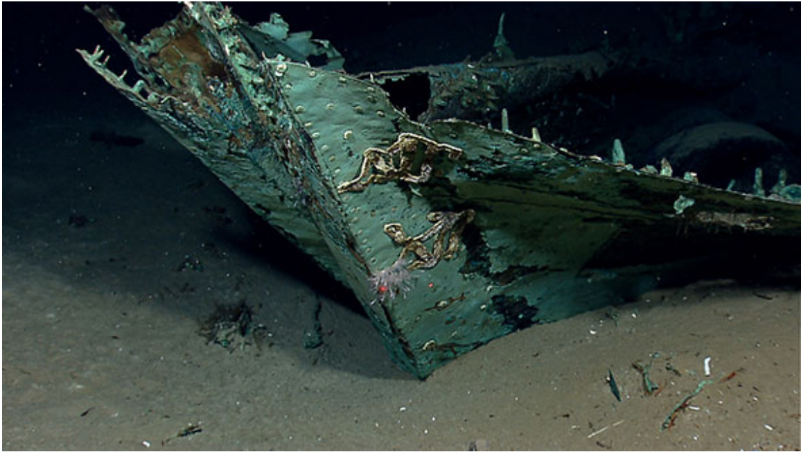
Figure C4. Copper sheathing covers the stern post of Monterrey A. Image credit: NOAA Okeanos Explorer Program.
