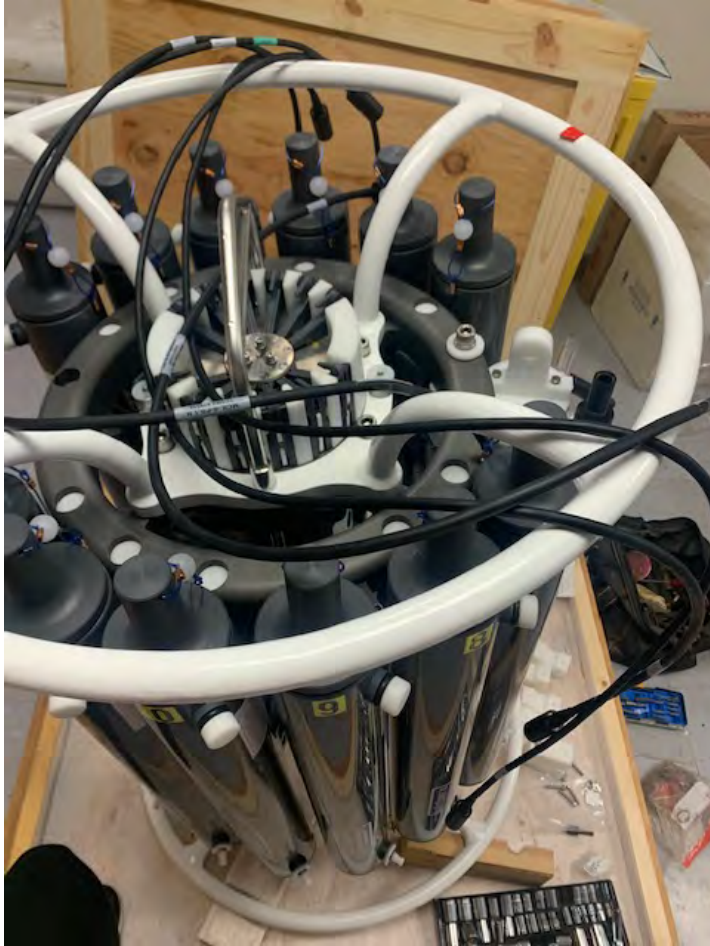
Figure 7. Replacement Seabird water quality carousel. Photo: O'Connell/NOAA
