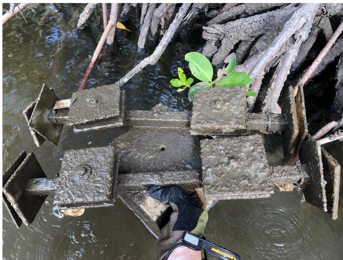
Figure 10. Settlement plates with high coverage of sediment on upper surface in May 2020
