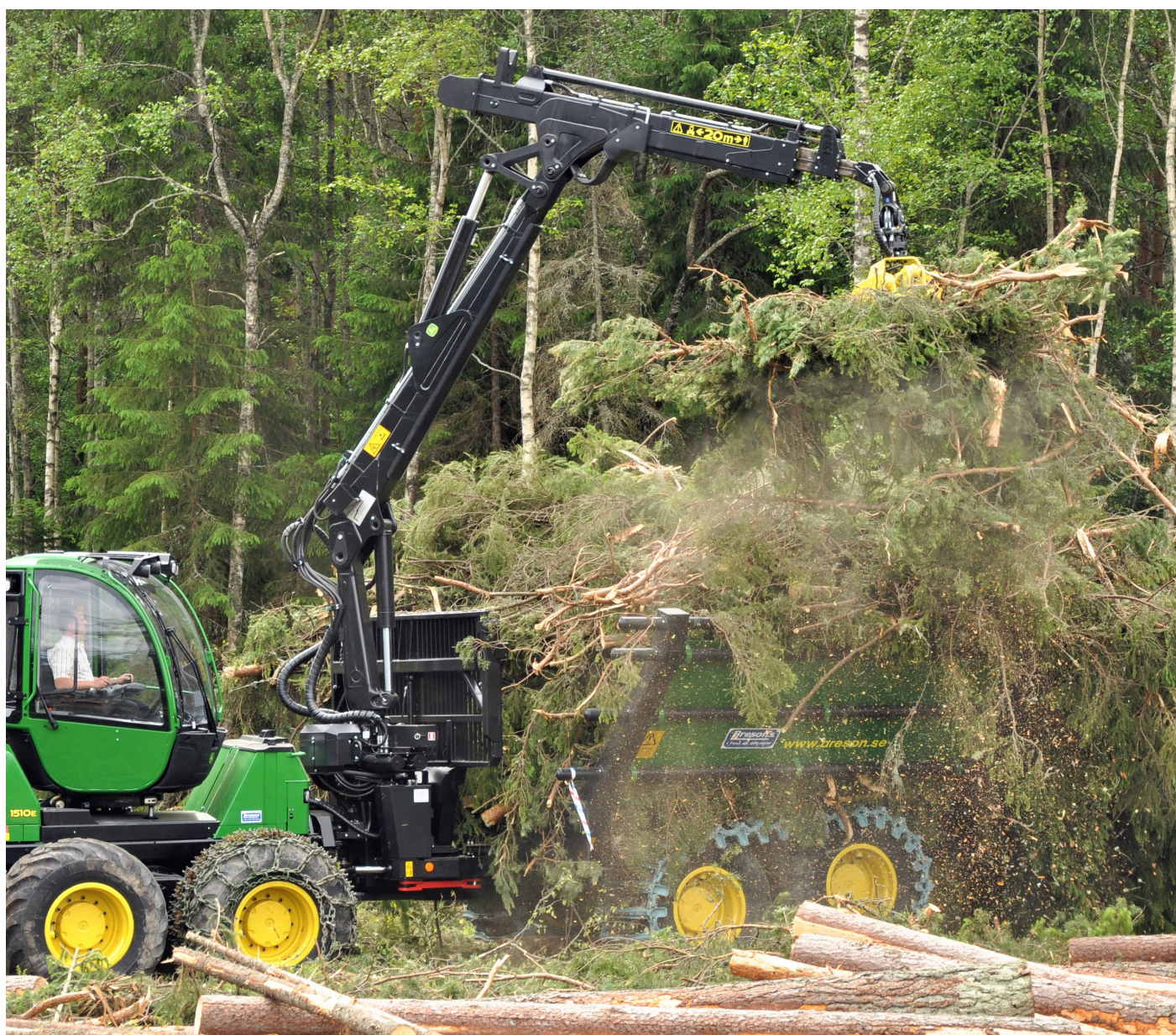
Figure 8. An intensified recovery of logging residues on suitable areas would greatly enhance the climate benefit of forestry. Forest chips substitute for fossil fuels, but logging residue is also a potential feedstock for various emerging bio-refineries.
