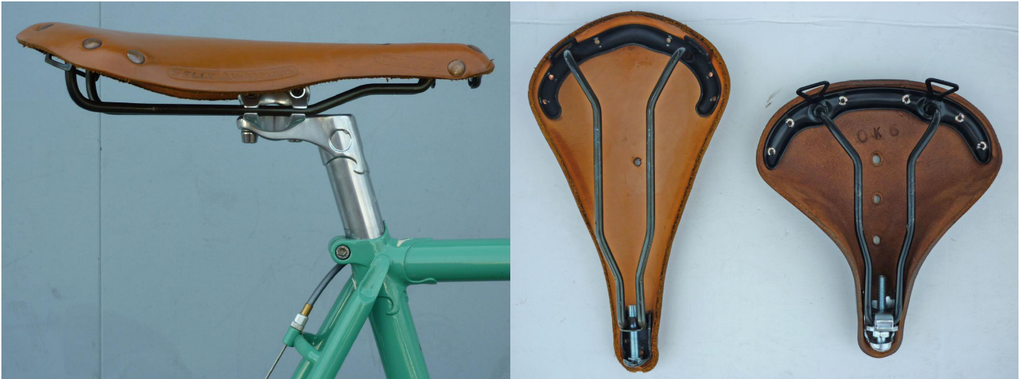
Lugged seat post and Selle Anatomica. Seat posts and saddles vary in how much you can shove the saddle back. This combo is the all-time champ.
