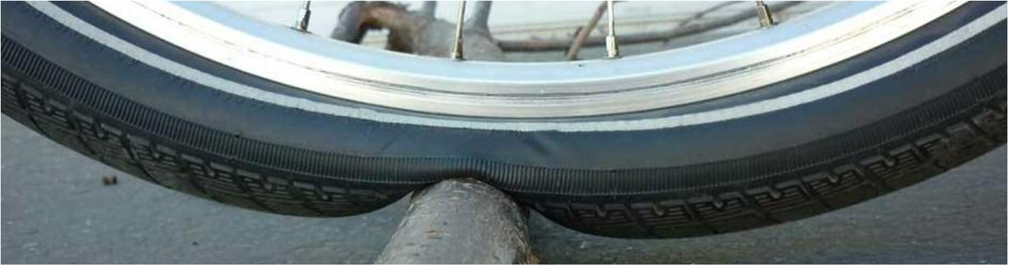
The oldest and least sophisticated form of bike shock-absorption, the big pneumatic tire.
