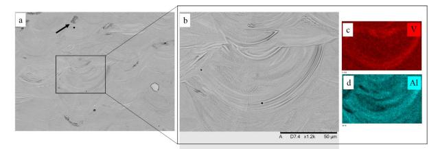
Figure 5: Backscatter SEM/EDS showing the general microstructural features of the sample built from simply mixed 2 feedstock.
