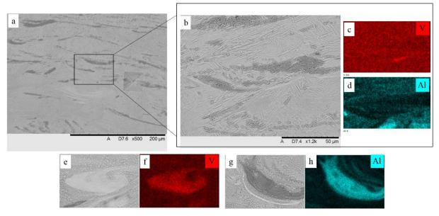
Figure 4: Backscatter SEM/EDS showing the general microstructural features of the sample built from simply mixed 1 feedstock.
