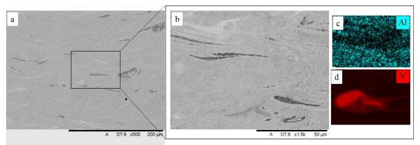
Figure 6: Backscatter SEM/EDS showing the general microstructural features of the sample built from satellited feedstock.
