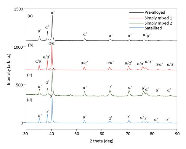
Figure 3: Comparison of the XRD spectra obtained from samples deposited from the: a) pre-alloyed, b) and c) simply-mixed, and c) satellited powder feedstocks.
