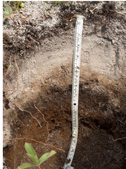
Soil profile of upland heath, showing eluviation in surface horizons and shallow rooting depth PHOTOS: L&F (Sean Basquill)
