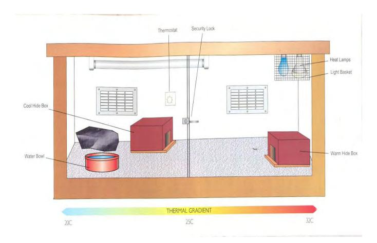
Hear a simple layout of an enclosure with the thermogradient. Notice a hide is provided at both ends of the gradient with the thermostat placed in the center.
