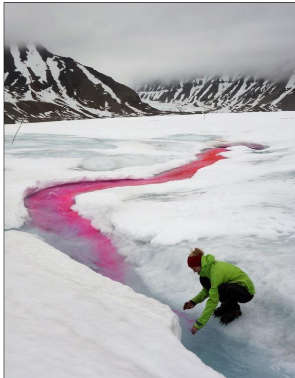
Figure 3.5: Injecting dye into the supraglacial stream upstream of moulin B, which is still hidden under a solid snow bridge. Photo: Myreng 2014.
