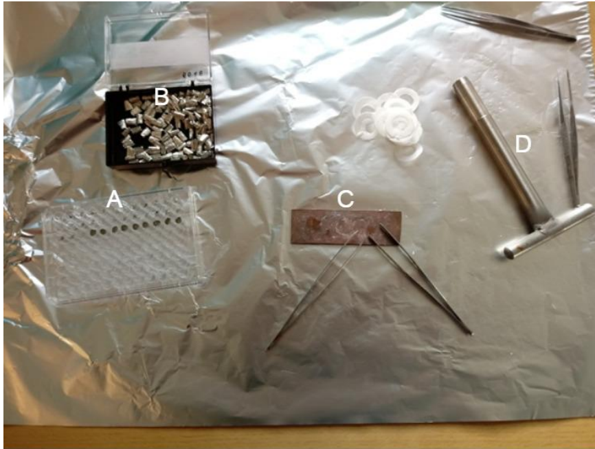
Figure 23 – The setup for preparing carbon samples. A a 96- well plate, B tin capsules, C metal board and tweezers, D the tool used to puncture the filters.
