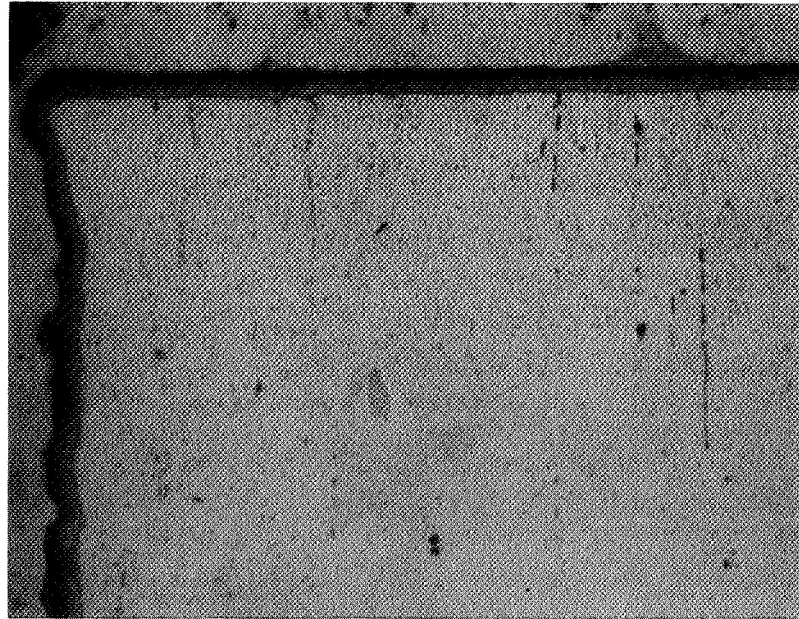
FIGURE 9: OPTICAL MICROGRAPH OF CROSS SECTION OF CHROMIUM ALLOY Cr-7Mo-2Ta-0.09C-0.1Y SHOWING CHROMIUM BORIDE LAYER Etched Electrolytically in a Solution of Sodium Hydroxide. Magnification 250X
