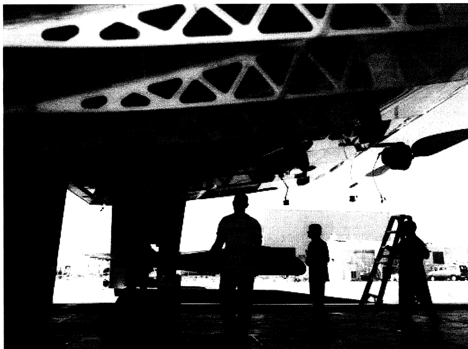
Dryden Flight Research Center EC96-43765-8 Photographed November 1996 LIGHT AS A FEATHER--Technicians easily lift a 20-foot wing section during assembly of the pathfinder solar-powered aircraft. NASA photo by Dennis Taylor
