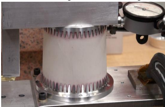
FIGURE 10: Lateral pull test thrust tube assembly
