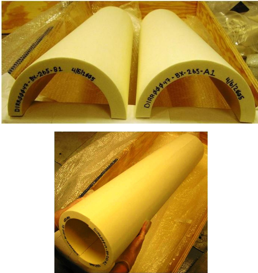
Figure 5. One of five 1-m long cylindrical clam shell test articles were produced for testing using a cylindrical thermal conductivity test instrument (Cryostat-100). Machined thickness of approximately 25-mm is shown in the top view while the precise longitudinal fit-up is shown in the bottom view.
