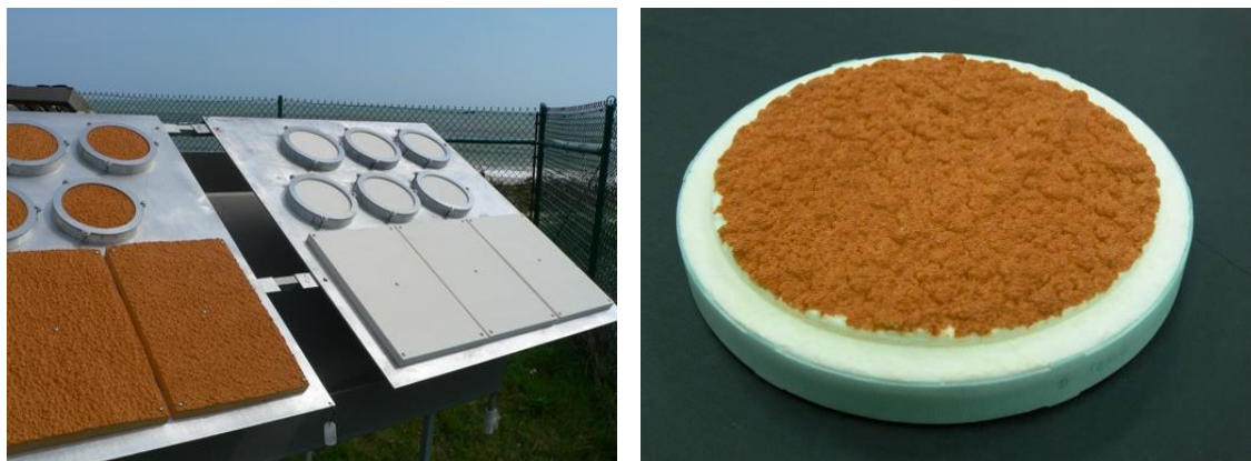
Figure 4. Weathering of SOFI test specimens exposure testing at the Corrosion Beach Site of the Kennedy Space Center (left). A one-month weathered specimen is shown on the right.
