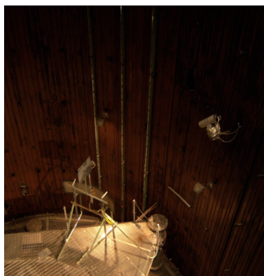
Figure 4: The simulated test article installed in the vacuum chamber. Three (3) vertical infrared lamp arrays are visible along the back wall.
