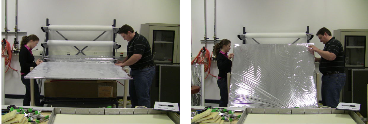
Figure 4. MLI Quick Layup Technique
