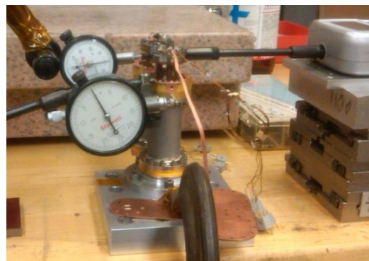
FIGURE 11: Lateral pull test heat switch 3 and 4
