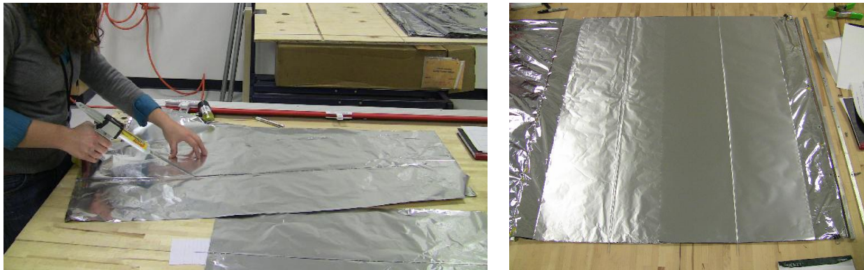
Figure 5. BAC Panel Layup Process
