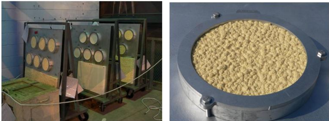
Figure 3. Aging of SOFI test specimens inside the Vehicle Assembly Building at Kennedy Space Center (left). The mounting enclosure is shown on the right.
