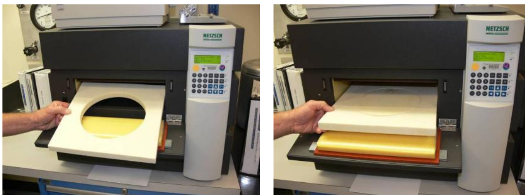
Figure 9. Specimen holding frame for heat flux meter testing (left); test specimen being installed for testing (right).
