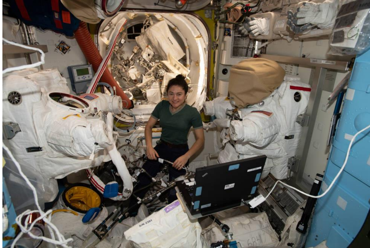
Fig. 3 PLSS on Suit Stand in Quest Equipment Lock
