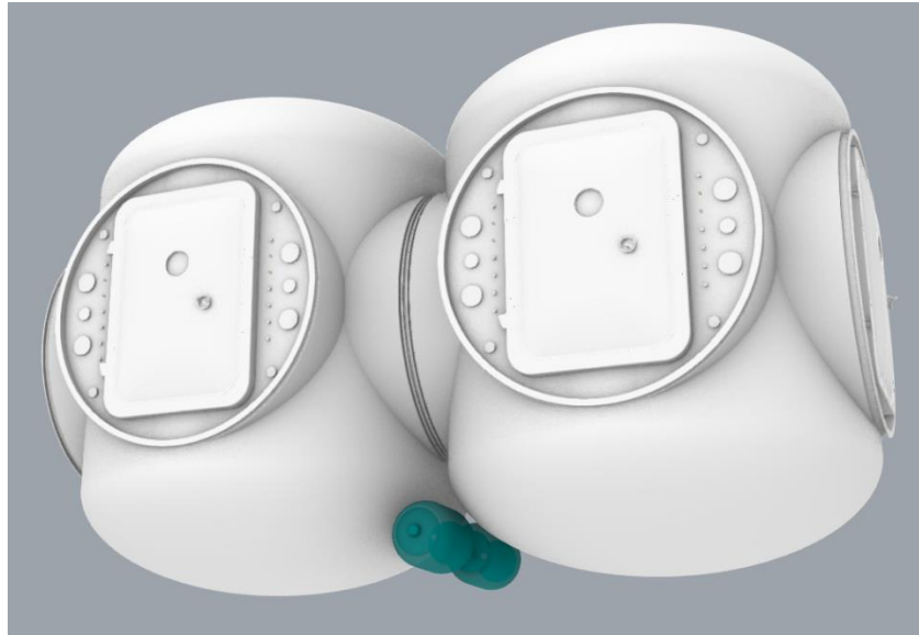
Fig. 28 TCAN Nitrogen and Oxygen Tanks
