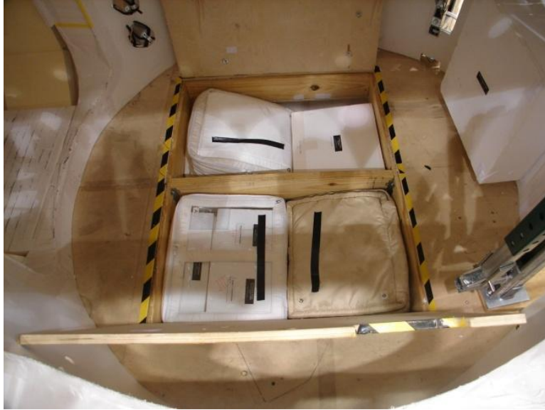
Fig. 7 Under-Floor Stowage in the Altair Airlock Mockup
