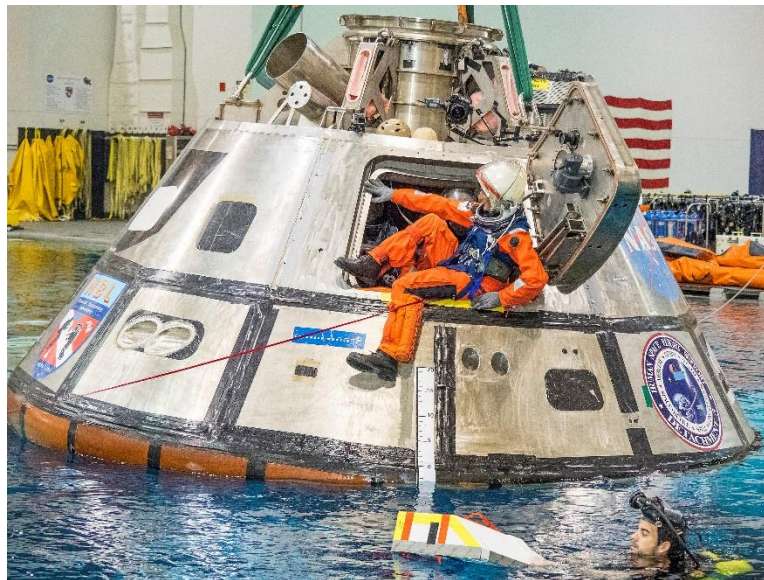
Fig. 23 Orion Mockup During Water Egress Testing
