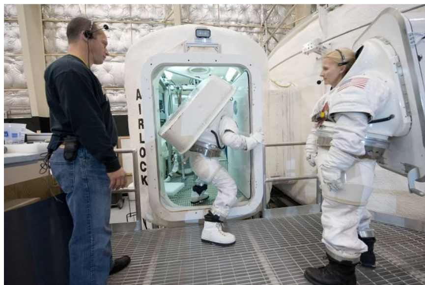
Fig. 21 Suited Crew Member Translation Through 40-inch by 60-inch Hatch
