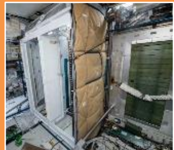
MCTBs deployed to adsorb treadmill noise
