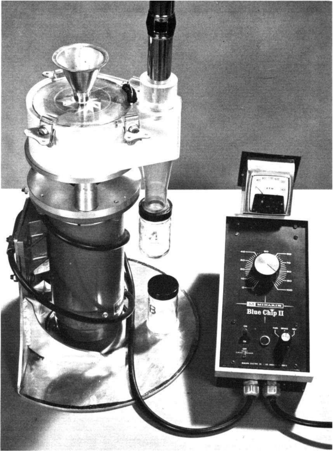
Figure 2. Mill with drive and speed controller.
