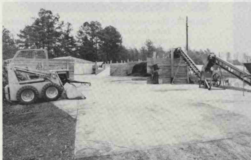
Figure 58. Media storage and preparation area is critical in the prevention of contamination by pathogens. A slightly raised concrete pad is ideal (R. K. Jones, NCSU).
