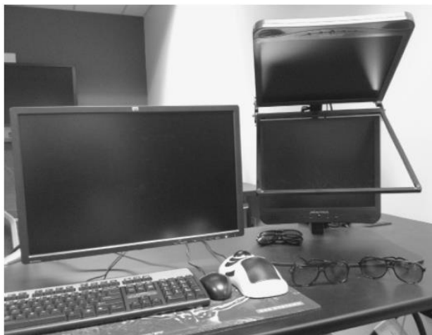
Figure 12-13. Softcopy photogrammetric workstation with polarizing filter stereo imaging. (Courtesy BAE Systems.)
