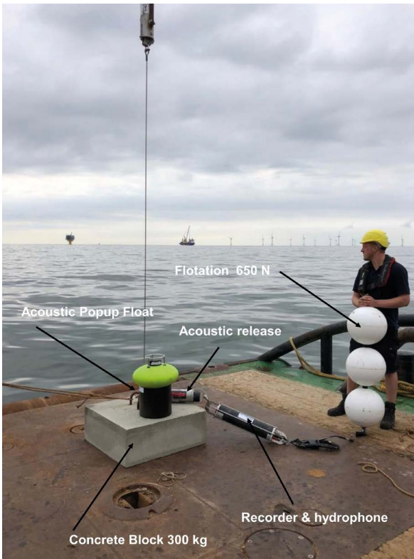
Figure 1. Mooring design of the underwater sound measurement equipment. Here on the rear deck of Zeetijger prior deployment.
