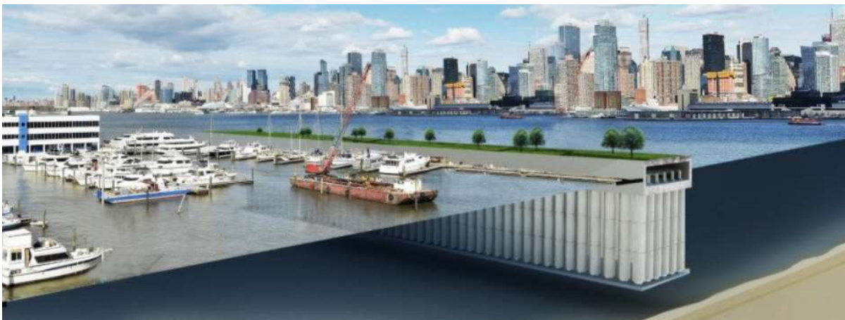
Waterstudio – Floating breakwater that harvests power for electricity from wave action.
