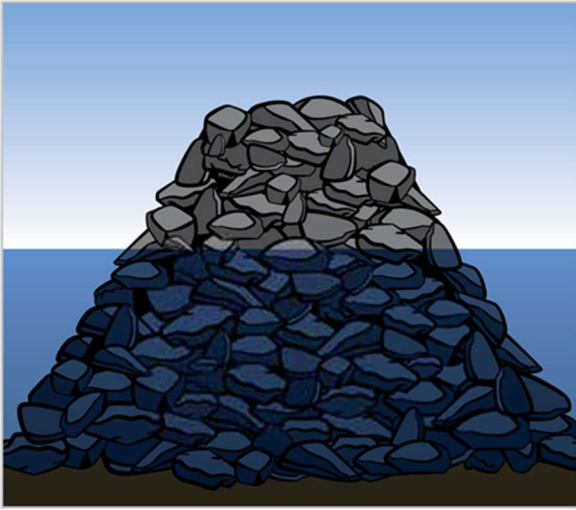
Rock jetties have a wide base on the ocean floor.
