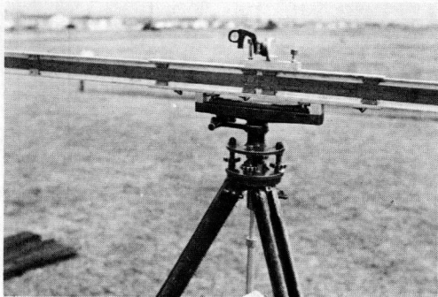
Figure 1. 10-ft subtense bar; leveling and sighting arrangement.
