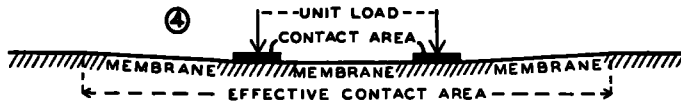
Figure B. Deconcentration of Total Load By Increasing Effective Contact Area By Means of Membrane. (Same Total Load as in Fig. A)
