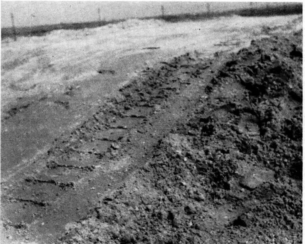
Figure 27. Soil surface pattern before dynamic compaction (at right) and after (at left) with Compactor B of nonconfined, cohesive silt-gravel sand (7 percent M.C.)
