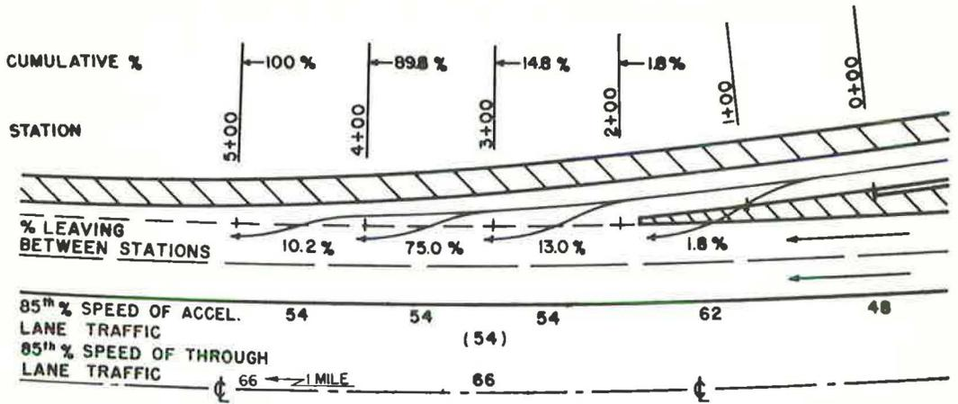
Figure 7. Speeds and lateral placement of passenger cars on type 1 acceleration lane, location Ale—Indiana Toll Road, LaPorte Interchange, westbound traffic.
