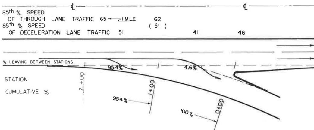
Figure 31. Speeds and lateral placement of passenger cars on type 3 deceleration lane, location D3a—Interstate 74, S. R. 9 Interchange, eastbound traffic.
