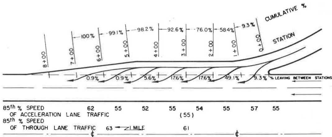
Figure 12. Speeds and lateral placement of passenger cars on type 2 acceleration lane, location A2c—Interstate 74, Post Road Interchange, eastbound traffic.
