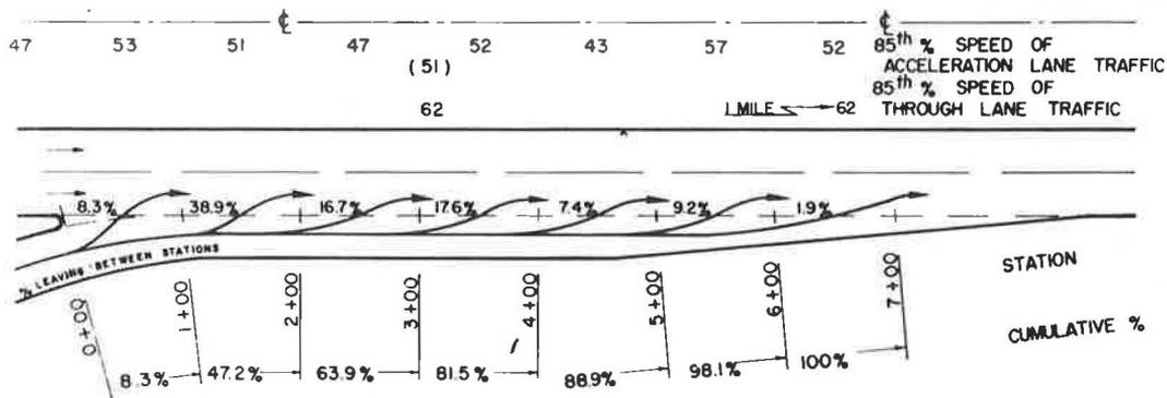
Figure 11. Speeds and lateral placement of passenger cars on type 2 acceleration lane, location A2b—Tri-State Highway, Kennedy Avenue Interchange, eastbound traffic.
