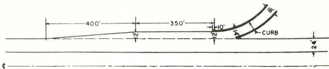
Figure 9. Acceleration lane, type 2.
