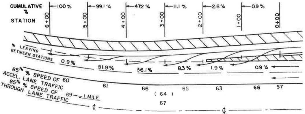
Figure 6. Speeds and lateral placement of passenger cars on type 1 acceleration lane, location Ald—Indiana Toll Road, Valparaiso Interchange, westbound traffic.
