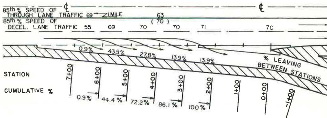
Figure 22. Speeds and lateral placement of passenger cars on type 1 deceleration lane, location D1a—Indiana Toll Road, Gary West Interchange, eastbound traffic.
