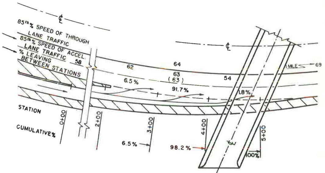
Figure 8. Speeds and lateral placement of passenger cars on type 1 acceleration lane, location Alf—Indiana Toll Road, Gary East Interchange, eastbound traffic.
