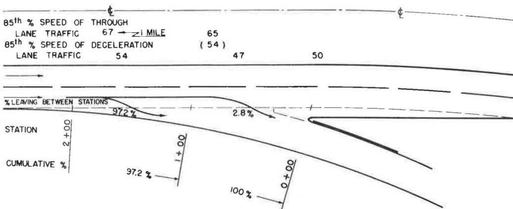
Figure 32. Speeds and lateral placement of passenger cars on type 3 deceleration lane, location D3b—Interstate 65 and S. R. 334 Interchange, southbound traffic.
