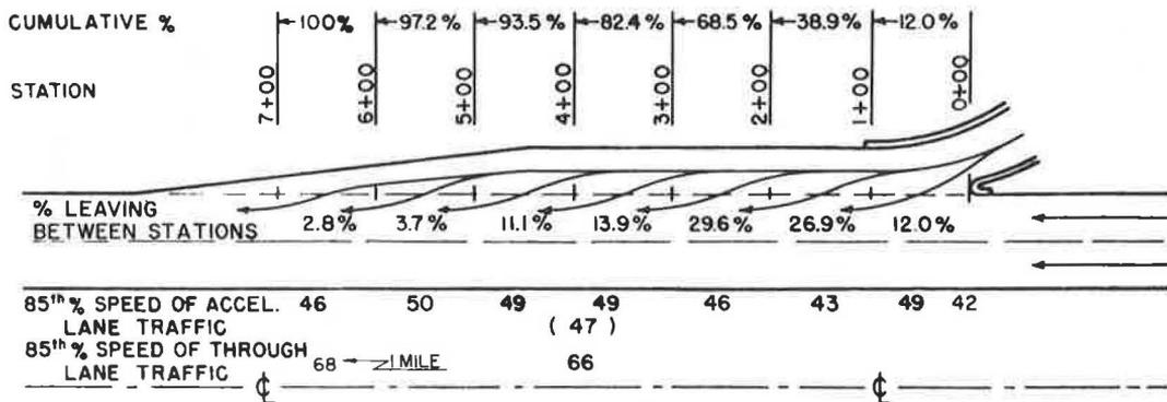
Figure 10. Speeds and lateral placement of passenger cars on type 2 acceleration lane, location A2a—Interstate 65, S. R. 39 Interchange, northbound traffic.
