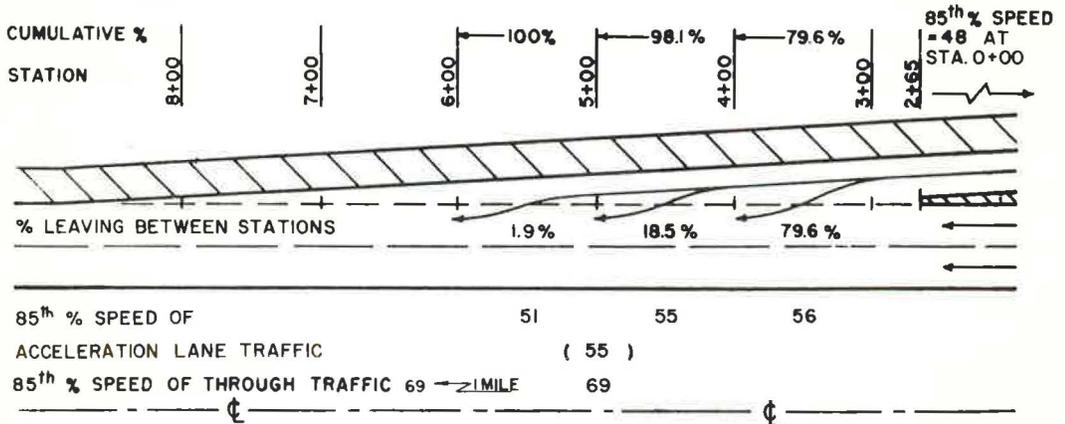
Figure 3. Speeds and lateral placement of passenger cars on type 1 acceleration lane, location A1a—Indiana Toll Road, Middlebury Interchange, westbound traffic.
