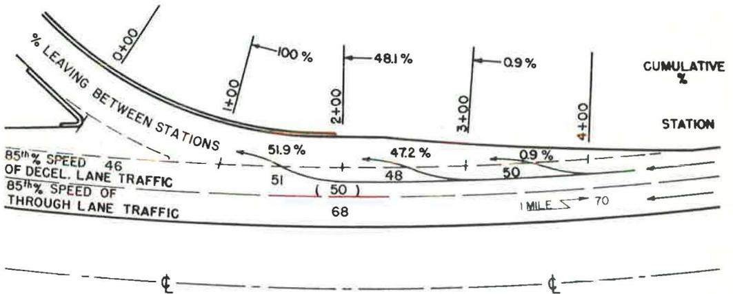
Figure 29. Speeds and lateral placement of passenger cars on type 2 deceleration lane, location D2c—Interstate 65, State Route 39 Interchange, northbound traffic.
