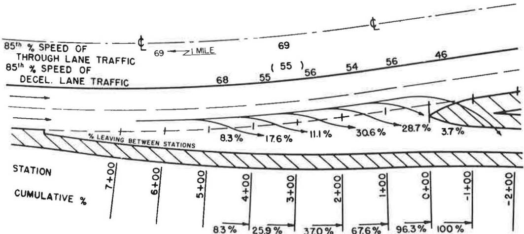
Figure 24. Speeds and lateral placement of passenger cars on type 1 deceleration lane, location Dlc—Indiana Toll Road, Chesterton-Valparaiso Interchange, eastbound traffic.
