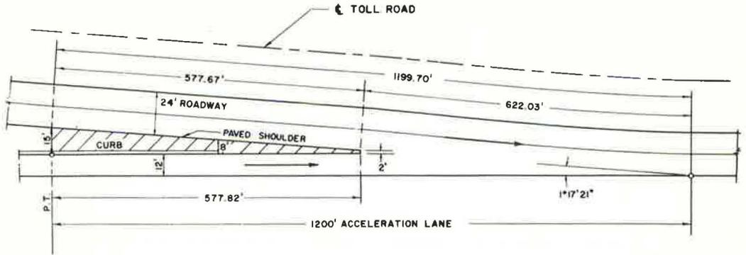
Figure 2. Acceleration lane, type 1.
