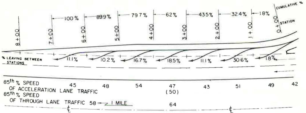
Figure 13. Speeds and lateral placement of passenger cars on type 2 acceleration lane, location A2d—Interstate 65, S. R. 60 Interchange, southbound traffic.
