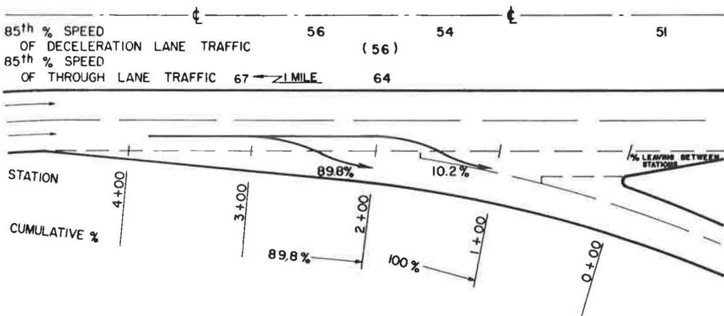
Figure 40. Speeds and lateral placement of passenger cars on type 5 deceleration lane, location D5b—Interstate 65 and S. R. 56 Interchange, northbound traffic.
