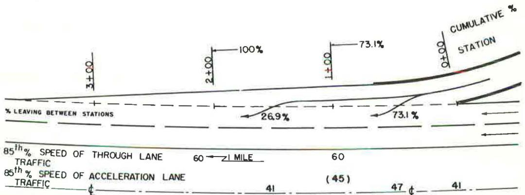
Figure 20. Speeds and lateral placement of passenger cars on type 4 acceleration lane, location A1b—Tri-State Highway, Calumet Ave. Interchange, westbound traffic.
