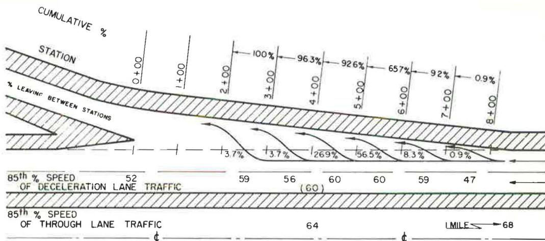
Figure 23. Speeds and lateral placement of passenger cars on type 1 deceleration lane, location D1b—Indiana Toll Road, Michigan City Interchange, westbound traffic.
