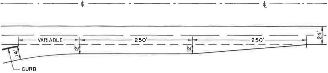
Figure 15. Acceleration lane, type 3.
