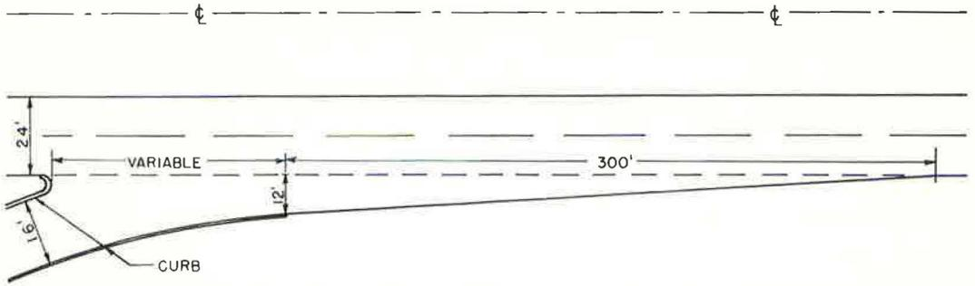
Figure 18. Acceleration lane, type 4.
