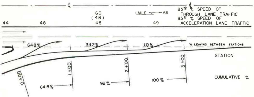
Figure 19. Speeds and lateral placement of passenger cars on type 4 acceleration lane, location A1a—Tri-State Highway, Calumet Ave. Interchange, eastbound traffic.
