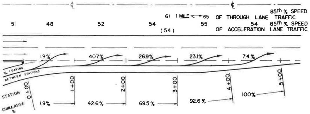
Figure 16. Speeds and lateral placement of passenger cars on type 3 acceleration lane, location A3a—Interstate 65, S. R. 56 Interchange, northbound traffic.
