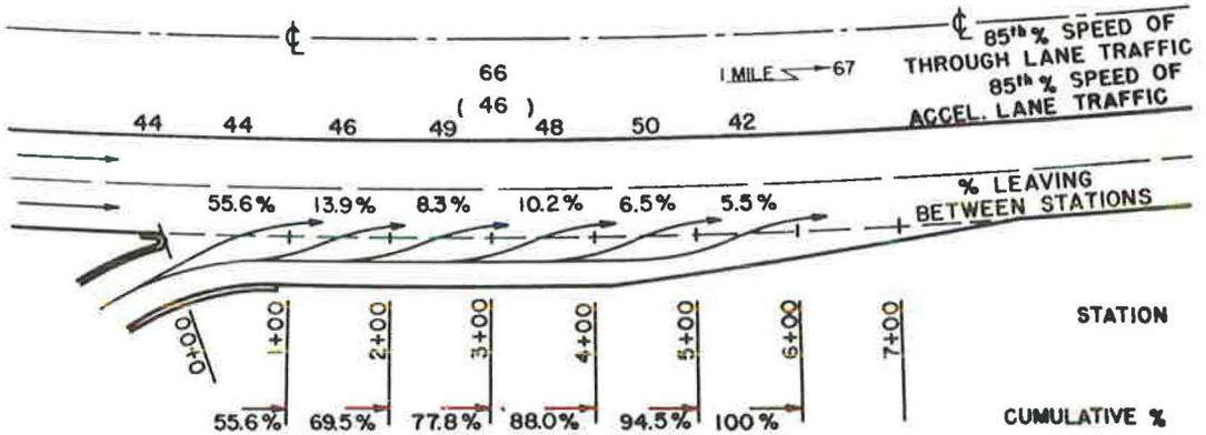
Figure 14. Speeds and lateral placement of passenger cars on type 2 acceleration lane, location A2e—Interstate 65, S. R. 39 Interchange, southbound traffic.
