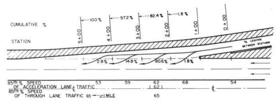
Figure 4. Speeds and lateral placement of passenger cars on type 1 acceleration lane, location Alb—Indiana Toll Road, Gary West Interchange, westbound traffic.
