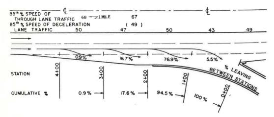
Figure 27. Speeds and lateral placement of passenger cars on type 2 deceleration lane, location D2a—Interstate 65, State Route 39 Interchange, southbound traffic.
