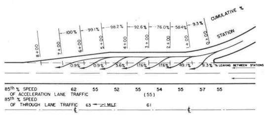
Figure 12. Speeds and lateral placement of passenger cars on type 2 acceleration lane, location A2c—Interstate 74, Post Road Interchange, eastbound traffic.
