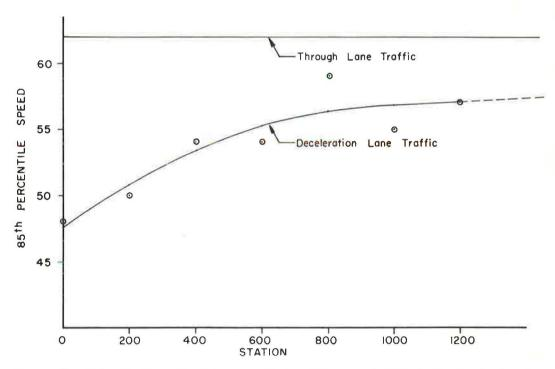
Figure 34. Determination of point where deceleration lane traffic begins to decelerate on through lane, location D3a.
