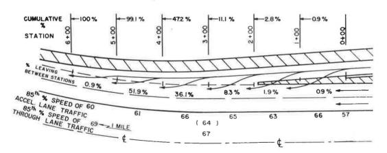
Figure 6. Speeds and lateral placement of passenger cars on type 1 acceleration lane, location Ald—Indiana Toll Road, Valparaiso Interchange, westbound traffic.
