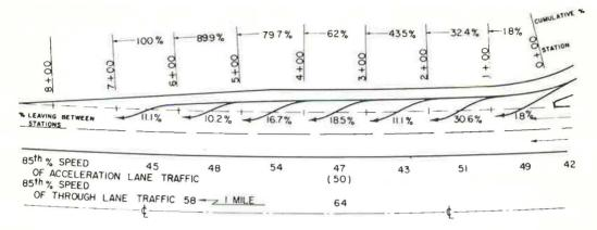
Figure 13. Speeds and lateral placement of passenger cars on type 2 acceleration lane, location A2d—Interstate 65, S. R. 60 Interchange, southbound traffic.
