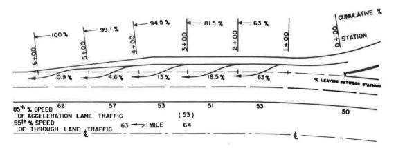
Figure 17. Speeds and lateral placement of passenger cars on type 3 acceleration lane, location A3b—Interstate 65, S. R. 334 Interchange, northbound traffic.
