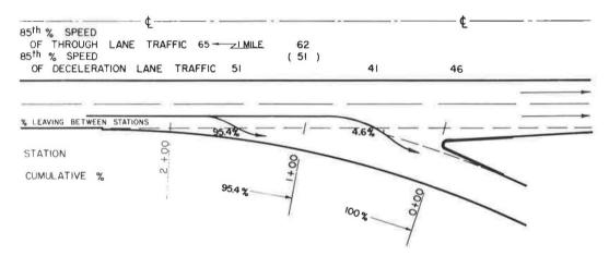
Figure 31. Speeds and lateral placement of passenger cars on type 3 deceleration lane, location D3a—Interstate 74, S. R. 9 Interchange, eastbound traffic.
