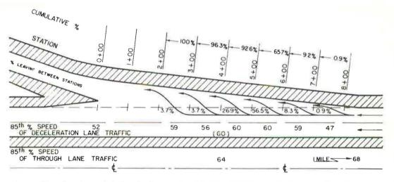
Figure 23. Speeds and lateral placement of passenger cars on type 1 deceleration lane, location Dlb—Indiana Toll Road, Michigan City Interchange, westbound braffic.
