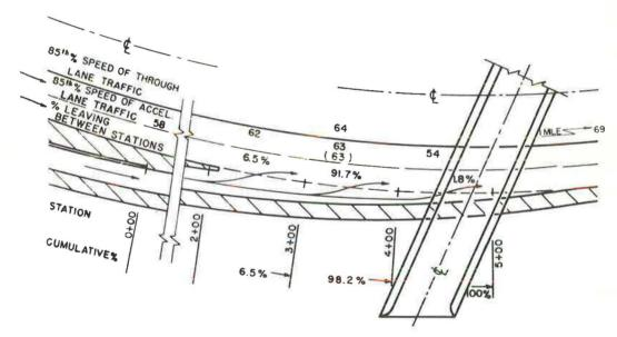
Figure 8. Speeds and lateral placement of passenger cars on type 1 acceleration lane, location Alf—Indiana Toll Road, Gary East Interchange, eastbound traffic.
