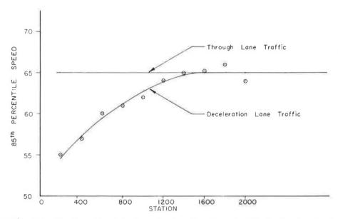
Figure 35. Determination of point where deceleration lane traffic begins to decelerate on through lane, location D3b.
