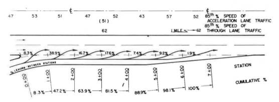
Figure 11. Speeds and lateral placement of passenger cars on type 2 acceleration lane, location A2b—Tri-State Highway, Kennedy Avenue Interchange, eastbound traffic.
