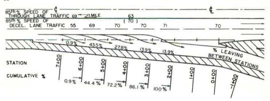
Figure 22. Speeds and lateral placement of passenger cars on type 1 deceleration lane, location Dla—Indiana Toll Road, Gary West Interchange, eastbound traffic.
