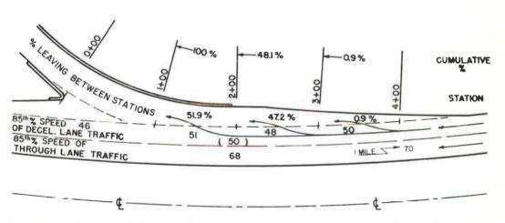
Figure 29. Speeds and lateral placement of passenger cars on type 2 deceleration lane, location D2c—Interstate 65, State Route 39 Interchange, northbound traffic.
