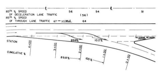
Figure 40. Speeds and lateral placement of passenger cars on type 5 deceleration lane, location D5b—Interstate 65 and S. R. 56 Interchange, northbound traffic.
