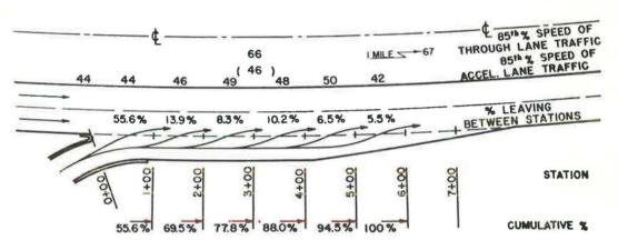
Figure 14. Speeds and lateral placement of passenger cars on type 2 acceleration lane, location A2e—Interstate 65, S. R. 39 Interchange, southbound traffic.
