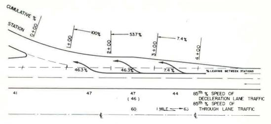
Figure 28. Speeds and lateral placement of passenger cars on type 2 deceleration lane, location D2b—Tri-State Highway and Kennedy Avenue Interchange, westbound traffic.
