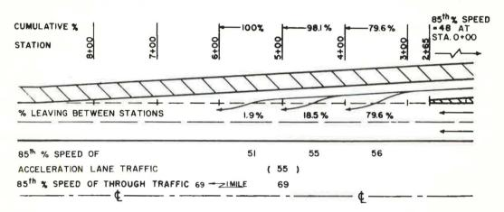
Figure 3. Speeds and lateral placement of passenger cars on type 1 acceleration lane, location Ala—Indiana Toll Road, Middlebury Interchange, westbound traffic.
