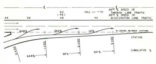
Figure 19. Speeds and lateral placement of passenger cars on type 4 acceleration lane, location A4a—Tri-State Highway, Calumet Ave. Interchange, eastbound traffic.
