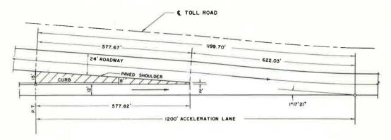
Figure 2. Acceleration lane, type 1.
