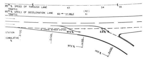
Figure 41. Speeds and lateral placement of passenger cars on type 5 deceleration lane, location D5c—Tri-State Highway and Calumet Avenue Interchange, eastbound traffic.
