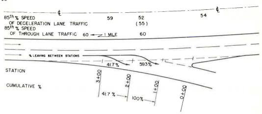
Figure 33. Speeds and lateral placement of passenger cars on type 3 deceleration lane, location D3c—Interstate 65 and S. R. 60 Interchange, northbound traffic.
