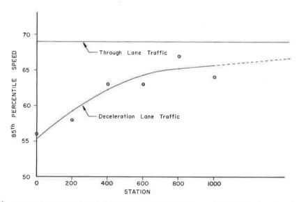
Figure 25. Determination of point where deceleration lane traffic begins to decelerate on through lane, location Dlc.
