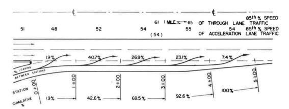
Figure 16. Speeds and lateral placement of passenger cars on type 3 acceleration lane, location A3a—Interstate 65, S. R. 56 Interchange, northbound traffic.
