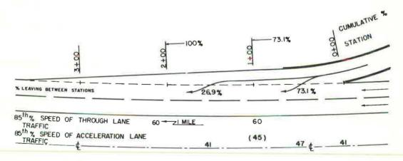
Figure 20. Speeds and lateral placement of passenger cars on type 4 acceleration lane, location A4b—Tri-State Highway, Calumet Ave. Interchange, westbound traffic.
