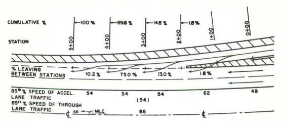
Figure 7. Speeds and lateral placement of passenger cars on type 1 acceleration lane, location Ale—Indiana Toll Road, LaPorte Interchange, westbound traffic.
