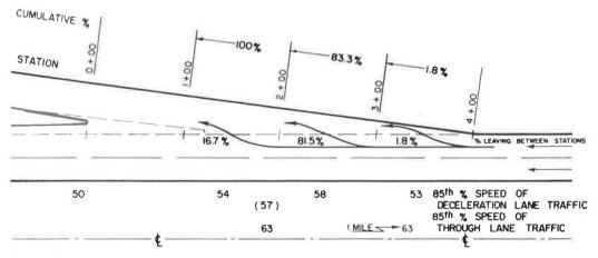
Figure 37. Speeds and lateral placement of passenger cars on type 4 deceleration lane, location D4a—Interstate 74, Pleasant View Interchange, eastbound traffic.
