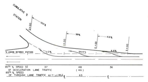
Figure 39. Speeds and lateral placement of passenger cars on type 5 deceleration lane, location D5a—Tri-State Highway and Calumet Avenue Interchange, westbound traffic.
