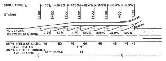
Figure 10. Speeds and lateral placement of passenger cars on type 2 acceleration lane, location A2a—Interstate 65, S. R. 39 Interchange, northbound traffic.
