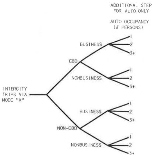
Figure 2. Procedure used to stratify intercity trips.
