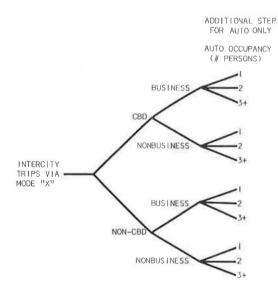
Figure 2. Procedure used to stratify intercity trips.
