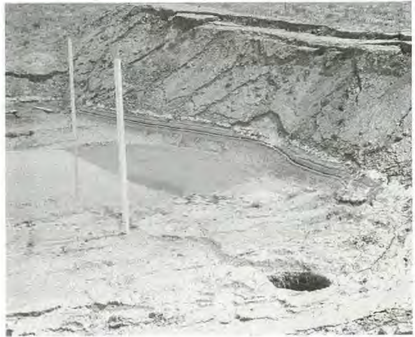
FIGURE 20-13 Results of saturation test on hydrocompactible colluvial soils in western Colorado; land surface has collapsed about 1 m.
