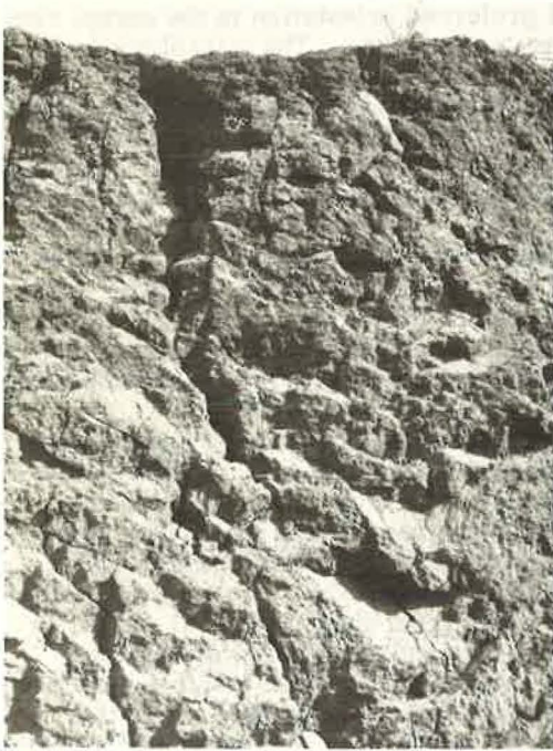
Figure 4. Vertisol profile showing wide cracking and common slickensides in a Vertisol; microhigh in upper right.
