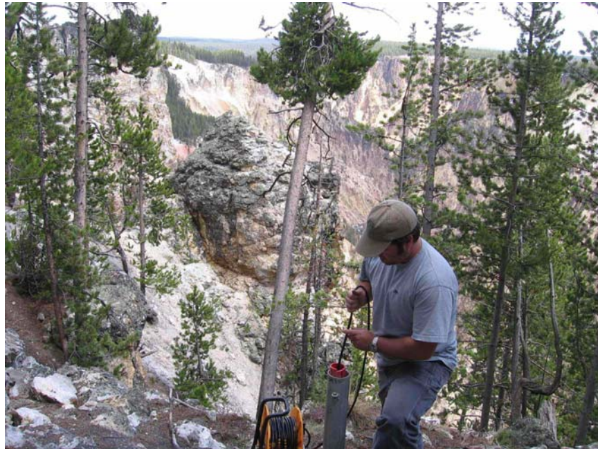
Inclinometer used for monitoring roadway stability in Yellowstone National Park (Beckstrand).
