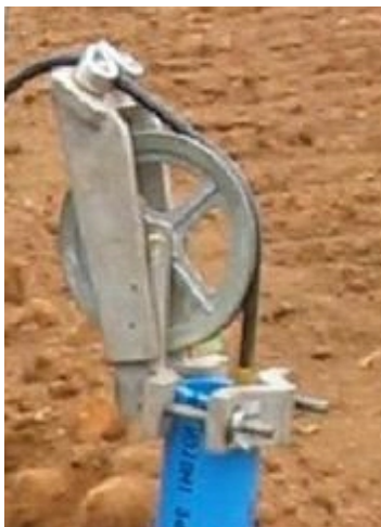
FIGURE 4 Cable control fixture.
