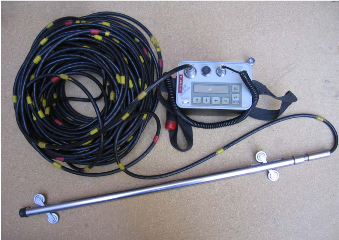
FIGURE 1 Typical inclinometer probe, cable, and readout device (Landslide Technology).
