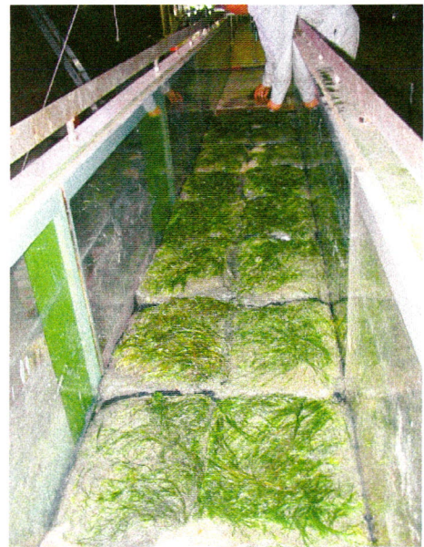
Natural sea grass vegetation ( Zostera Noltii ) in a wave flume of WL | Delft Hydraulics preceding a wave experiment.
