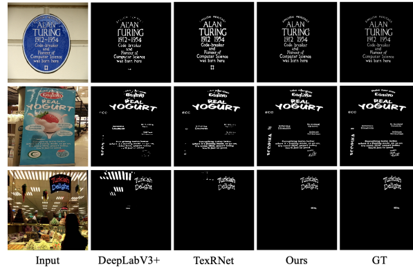
Fig. 7. Segmentation results for typical difficult samples. From top to bottom, each row is large variations in the scale and shape of text, scattered distribution of text throughout the image, and small text hidden in complex background noise, respectively.
