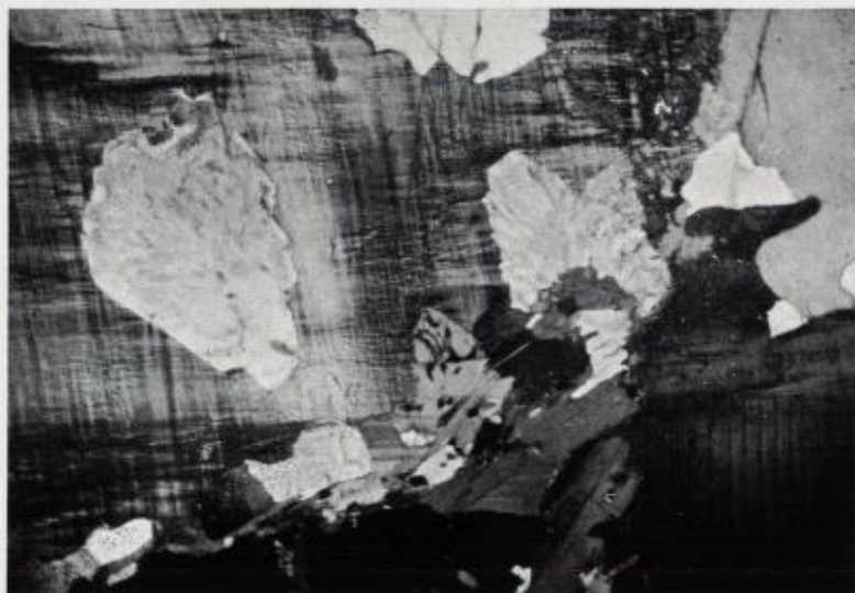
Fig. 14. Microphoto of microcline with inclusions of plagioclase and myrmekite. Granite, N of Kiland, Åmli. \times 18 , nic. crossed.
