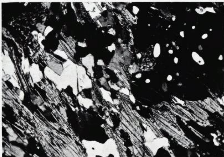
Fig. 3. Microphoto of sillimanite gneiss. Skutterud, Modum. \times 18 , nic. crossed (microcline-perthite, quartz, sillimanite, biotite).
