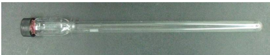
Figure 3.13: NMR tube for the setup of ALTADENA and PASADENA under pressure.
