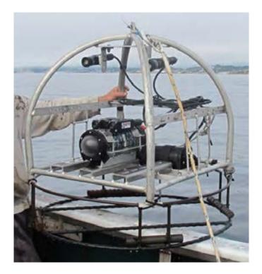
Figure 8. Video lander, showing the camera pressure tube, lasers, lights, and battery pressure tube mounted within the aluminum frame.
