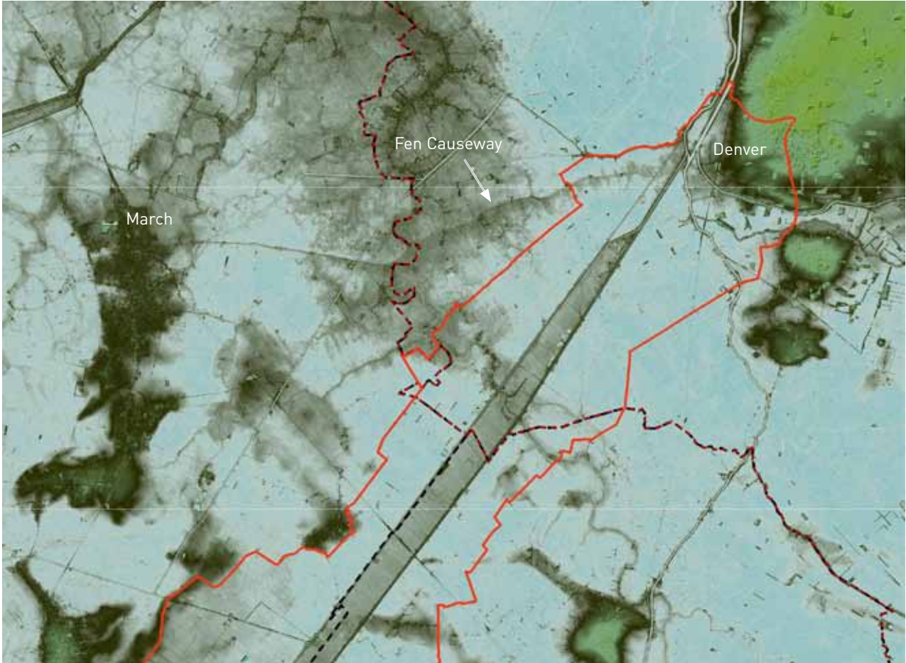
The route of the Roman Fen Causeway is visible on the digital terrain model as a band of silt running broadly east-west across the fen between March and Denver
