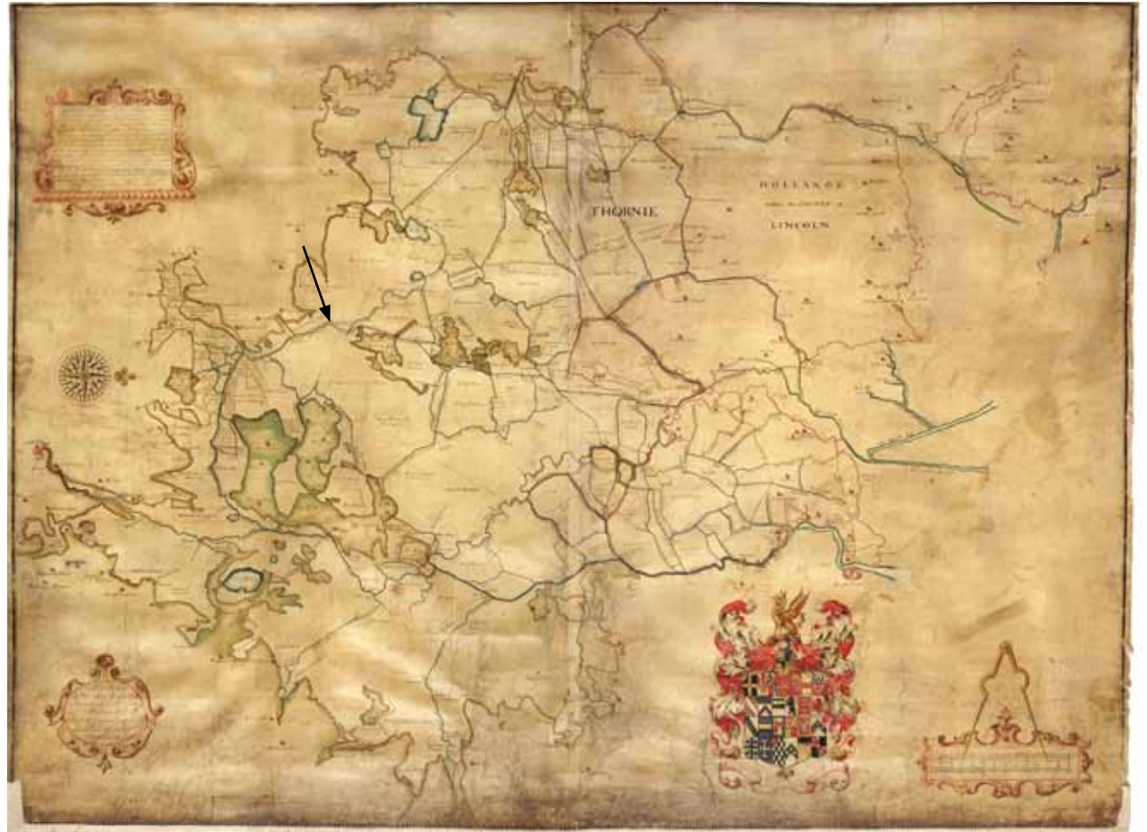
"An Exact Copy of A Plan of the Fens as it was taken Anno 1604 by William Hayward, carefully copy'd from ye Original". Plan of the Great level of the Fens, showing the pre-drainage water courses. Scale 1" to 1 mile. Not the original, but a 1727 copy by Payler-Smith. The original is not known to survive. Hand drawn on linen-backed paper. The black arrow indicates the alignment of the historic West Water. Ref. R59/31/40/1. Reproduced by kind permission of Cambridgeshire Archives.
