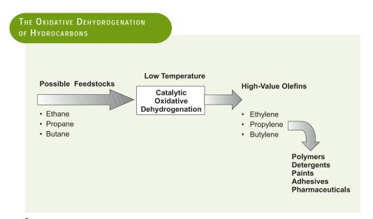
Low temperature catalytic process can replace energy-intensive steam cracking, producing high-value chemicals.
