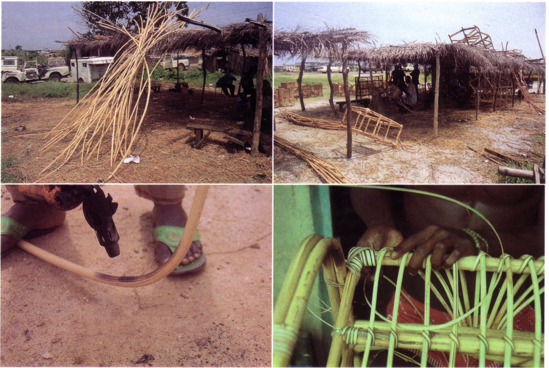
8 (Upper left). Laccosperma secundiflorum (the large diameter cane) drying in the sun after cleaning. 9 (Upper right). A typical rattan furniture workshop by the roadside in Lagos. 10 (Lower left). Laccosperma secundiflorum cane being bent to shape with a kerosene blow-lamp. 11 (Lower right). The frame of the chair made from L. secundiflorum . The joints are bound using "cane ropes" peeled from the stem of E. macrocarpa (the small diameter cane).
