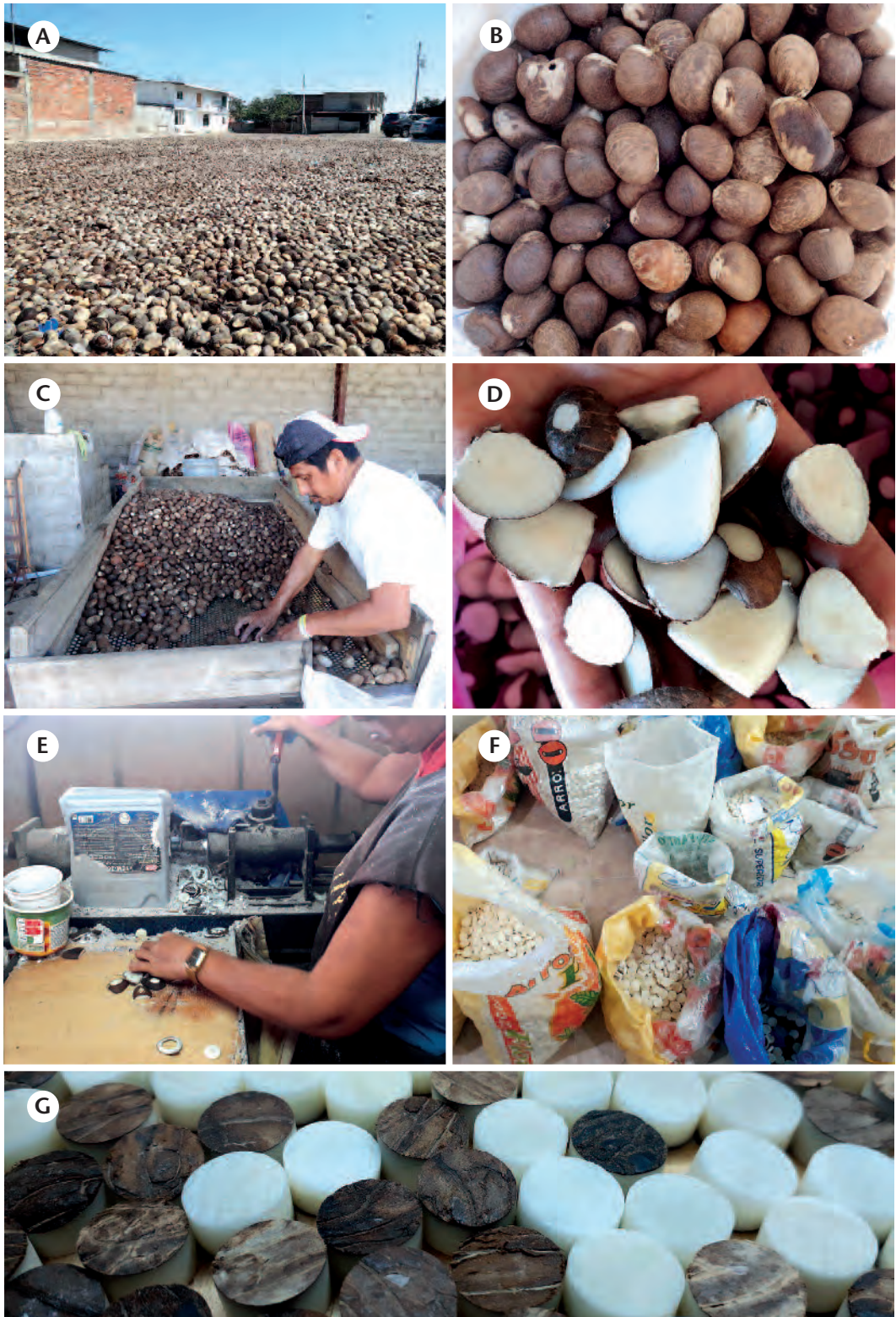
4. Production of animelas , the precursors of buttons, in the town of Manta. A. Drying of tagua seeds under the sun. B. Dried seeds. C. Selection of dried seeds according to their size. D. Slices resulting from the cut using a sawblade. E. Making of a hole in the slices. F. Resulting animelas sorted by size. G. Refined animelas conserving the pericarp of the tagua seeds. Photos by S. Escobar.
