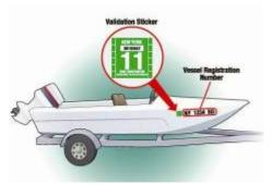
that contrasts with the hull color to enhance visibility. The registration number must be permanently attached; this means painted, decals, or stickers. There should be a space or dash between the letters and numbers: NY 1234 XY or NY-1234-XY.
