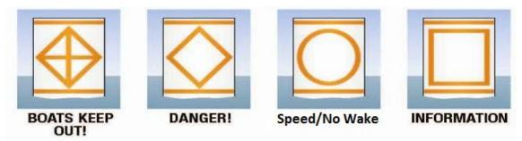
Waterways, just as roads, are marked to provide direction, advise caution, and to point out specific hazards. Understanding the waterway marking systems is important as these markers will assist in navigation, mark safe waters, and convey important information to the operator. There are two different navigational aid marking systems in use in the U.S, one for tidal and ocean waters, and one for inland waterways.
