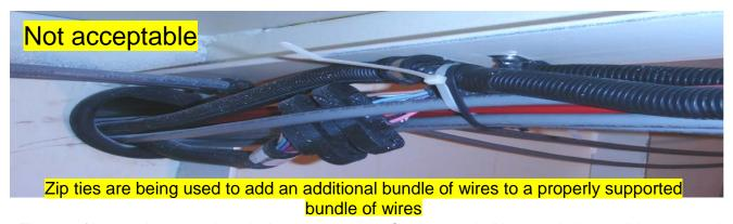
The use of house wire or speaker wire is not acceptable. Conductors shall be stranded, not solid, copper and must be labeled "marine" or "boat". For AC and especially for DC systems there are formulas you need to use when adding or replacing equipment on board. The Marine Services Bureau can assist you in determining the correct wire sizes.
