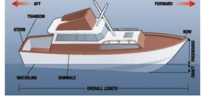
The draft determines the depth of water in which your boat can operate—the larger the draft, the deeper the water must be for the boat to operate without running aground.
