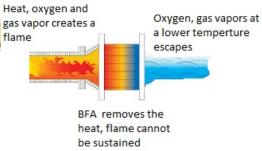
Check your arrestor periodically to ensure that it still fits snugly against the air intake. The arrestor should be removed and cleaned each season with de-greaser or soap and water to ensure that air flows into the engine properly.
