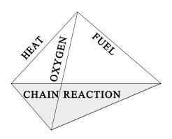
cannot exist or start if one of these four is missing. (As discussed in the section covering Backfire Flame Arrestors) Once started, a fire will grow in size and intensity at an increasing rate as long as all four elements are available. In order to extinguish a fire one or more of the elements represented by the tetrahedron's sides must be removed.
