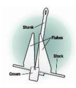
All Public Vessels must carry an anchor of an appropriate type, weight, and strength to hold the vessel securely during all weather conditions characteristic to the waterway upon which the vessel will operate.
