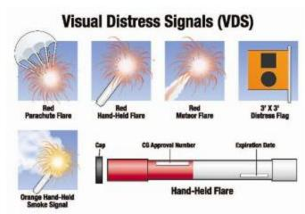
distress signals do not burn. Each type of distress signal has distinct advantages and disadvantages, and no single device is ideal under all conditions or suitable for all purposes.
