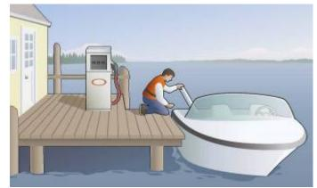
Don't overfill your tank! The tank will overflow and the spilled fuel will pose a fire hazard. Once you've filled the tank, open up all hatches. On an inboard boat, run the blower for at least 4 minutes to rid the boat of stray vapors. Fill portable tanks on the dock to keep gas vapors out of the boat.
