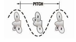
between the distance a propeller should move in one revolution through a solid medium and the actual distance it moves through water, a yielding substance. Picture a bicycle wheel moving over the pavement. Now picture it riding through a muddy field. The bicycle will move farther over pavement than it will through the mud—how much farther it moves is the slip.
