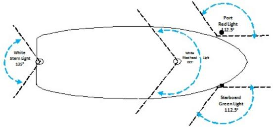
The type of lights your boat must have depends on the size and type of the boat.
