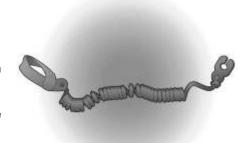
If the machine is equipped with a lanyard engine cut-off system, the lanyard must be attached to the operator and the shut off button. Many manufacturers of outboard engines and boats are adding cut-off systems as standard equipment.
