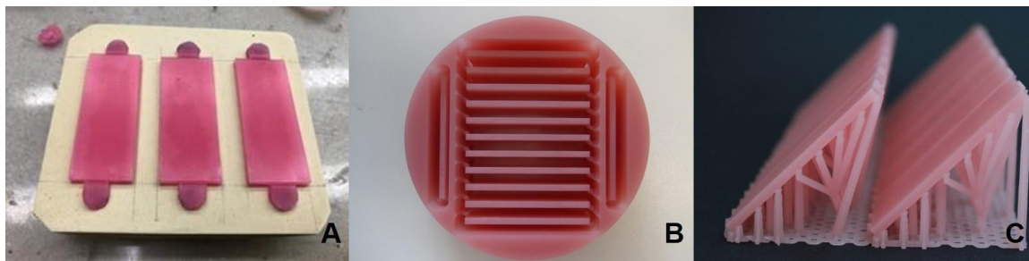
Figure 2. (A): Conventional specimens constructed in wax for further casting process. (B): Subtractively manufactured specimens in the polymethyl methacrylate (PMMA) block. (C): Additively manufactured specimens with the 45° printing orientation.
